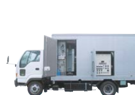
Mobile power generating system
