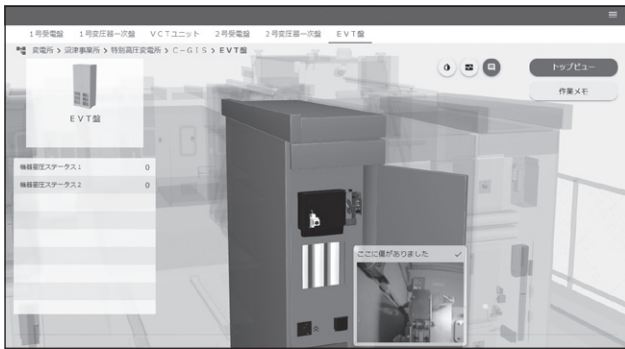
Fig. 6 Example of Information Sharing Using 3D Model
