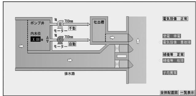
**Fig. 2** Pumping Station Monitoring Screen
