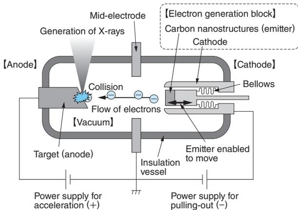
**Fig. 3 Outline of Newly Developed Cold Cathode X-ray Tube**
