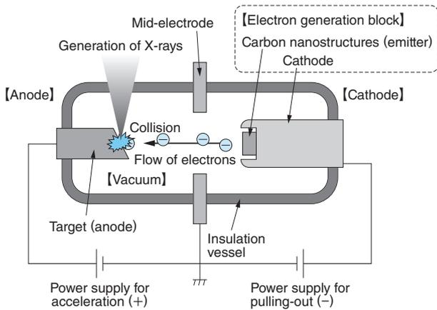
**Fig. 2 Outline of Cold Cathode X-ray Tube**
