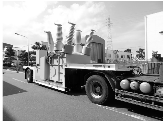
Fig. 5 Application Example of Mobile Switchgear
