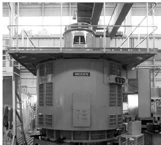
Fig. 5 Large Size Vertical Shaft-Wound Rotor Type Induction Motor
