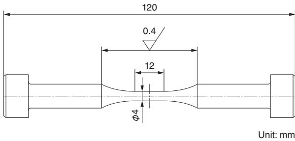
**Fig. 3 Specimen for Fatigue Test**
