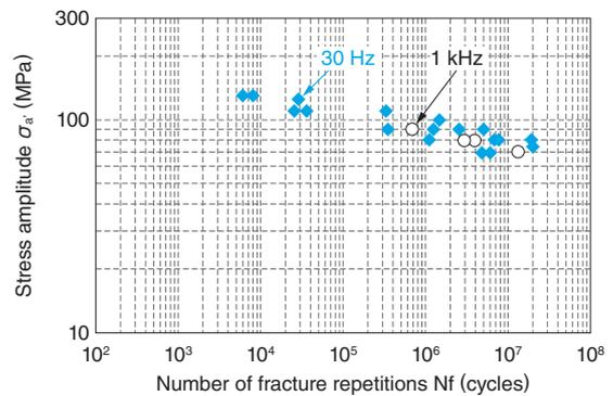
**Fig. 6 S-N Curve (Testing speed dependence)**
