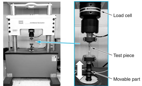
**Fig. 2 1 kHz Servohydraulic Fatigue Testing System**
