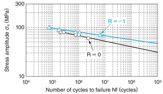
Fig. 7 S-N Curves with Stress Ratios  $R = -1$  and  $R = 0$
