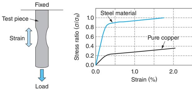
**Fig. 1 Stress-Strain Curves of Steel and Pure Copper**
