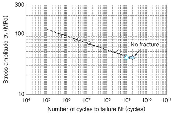
**Fig. 9 S-N Curve (Super-Long Life Region, R = 0, Room Temperature)**
