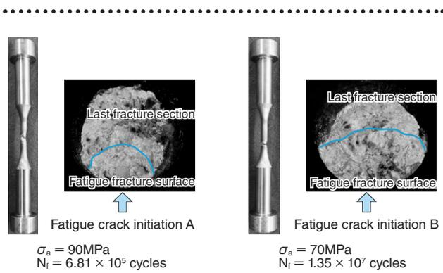
**Fig. 10 Fractured Test Piece and Fracture Section**
