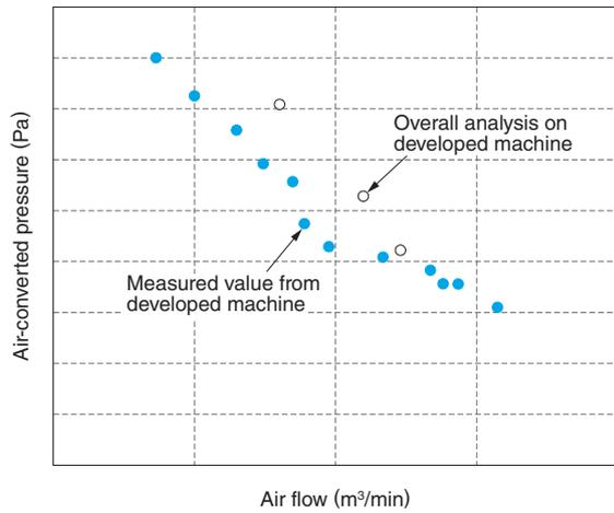
**Fig. 11 P-Q Curve of the Prototype**
