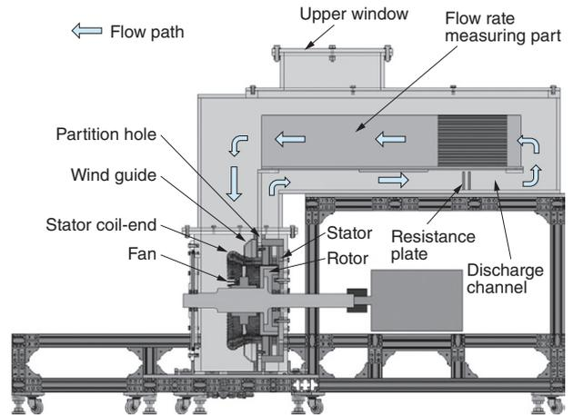
**Fig. 7** Outline of Smaller Model Experiment Equipment
