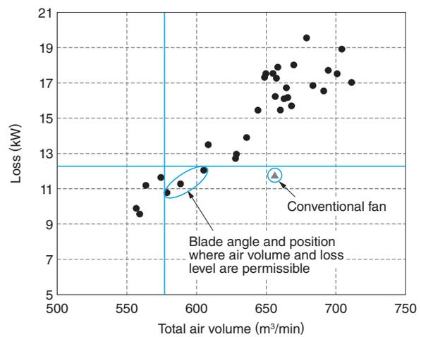
**Fig. 4 Study Result on Fan Blade Angle and Position**
