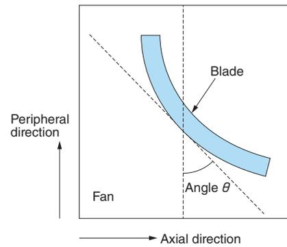
**Fig. 3 Definition of Blade Angle for a Fan**
