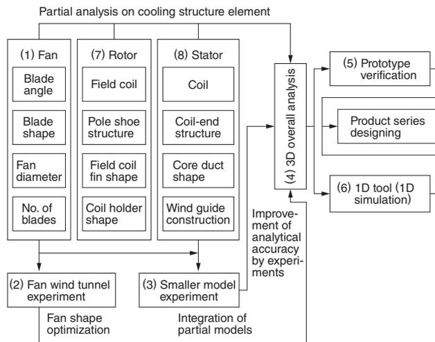
**Fig. 2 Workflow of New Structure Development Programs**
