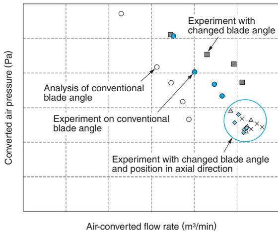
**Fig. 8 P-Q Curve Obtained from Smaller Model Experiments (by Prototype Conversion)**
