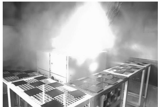
**Fig. 5** Situation of the Internal Arc Fault Test
