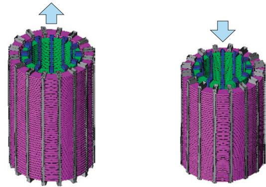
(a) Axial expansion/contraction mode for disc windings
