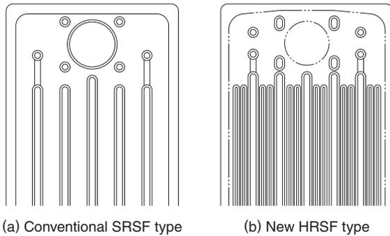
**Fig. 6 Comparison of Panel Shapes**
