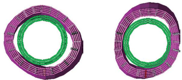
(b) Slantwise oval mode in radial direction for layer windings
