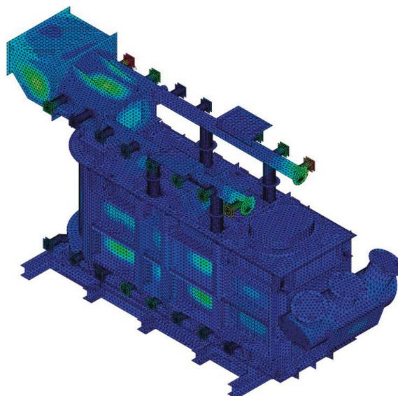
**Fig. 8** Result of Vacuum Durability Analysis
