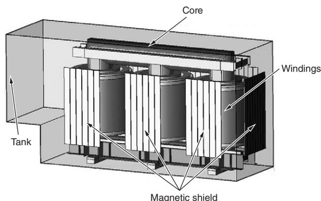
**Fig. 1 3D Model (Conventional Structure Design)**
