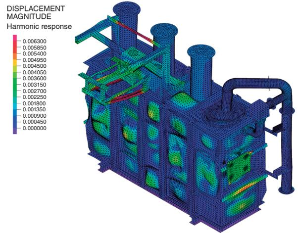
**Fig. 4** Result of Frequency Response Analysis on Actual Model
