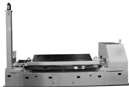
Fig. 3 AGV for Transporting Small-Sized Paper Rolls
