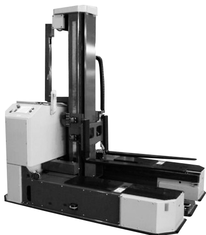
Fig. 4 AGV for Transporting Container
