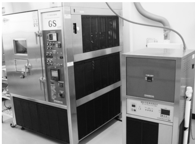
Fig. 1 Gas Corrosion Acceleration Test Equipment
