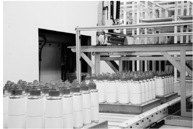
Fig. 10 VIs for Reclosers
