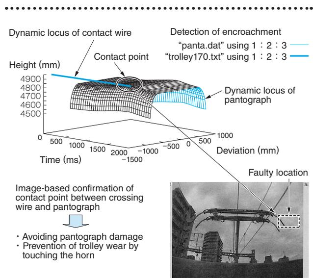
**Fig. 3 Static Wire Position Measurement and Detection of Crossing Wire Encroachment**
