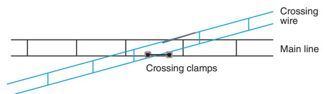
**Fig. 1** Outlined Diagram of Crossing Wires Section
