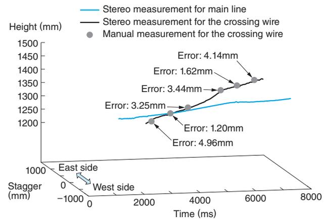
**Fig. 7** Result of Crossing Wire Measurement for Static Wire Position Measurement
