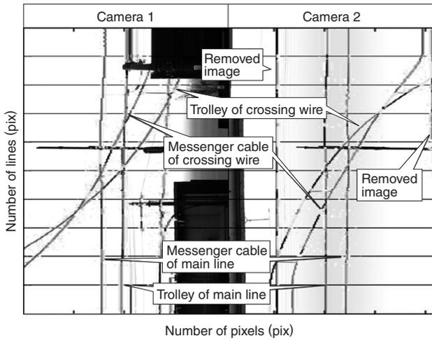
**Fig. 4** Result of Static Wire Position Measurement
