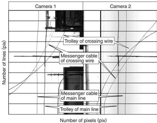
**Fig. 5** Original Image of Crossing Wire for Static Wire Position Measurement
