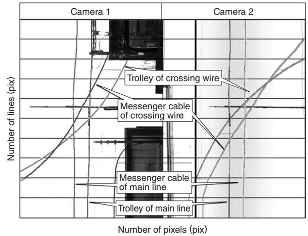
**Fig. 6** Result of Crossing Wire Measurement for Static Wire Position Measurement
