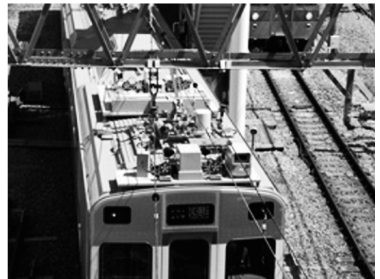
Fig. 2 Conventional Dedicated Inspection Car Equipped with the OCS System
