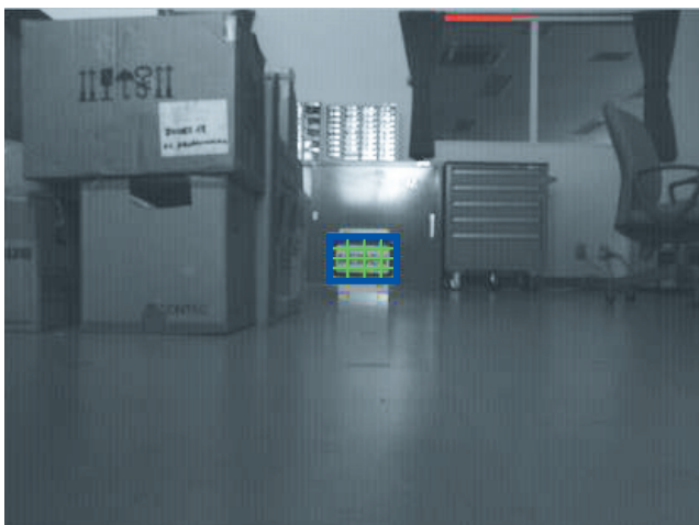
Fig. 6 Marker Detection Using Features in Closed Curve, Example 2
