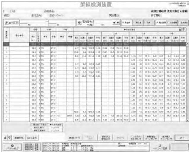
Fig. 5 Tabular Form Window Various reports specialized for each measurement items are available. Fig. 5 shows a sample report for wear measurement in tabular form.
