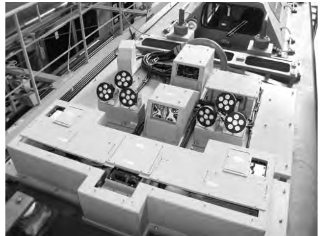
Fig. 4 FRP Cover for Rooftop Equipment
