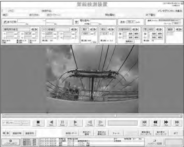
Fig. 7 Pantograph Monitoring Window This function provides a video replay of pantograph images by the CCD camera together with other measurement results as numerical values.
