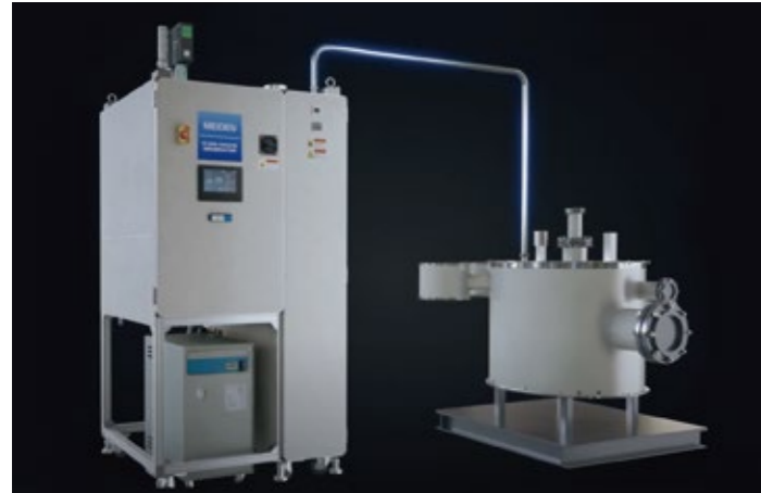
Connection image of POG and conventional ALD equipment
