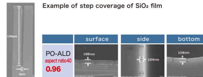
Example of step coverage of SiO 2 film
