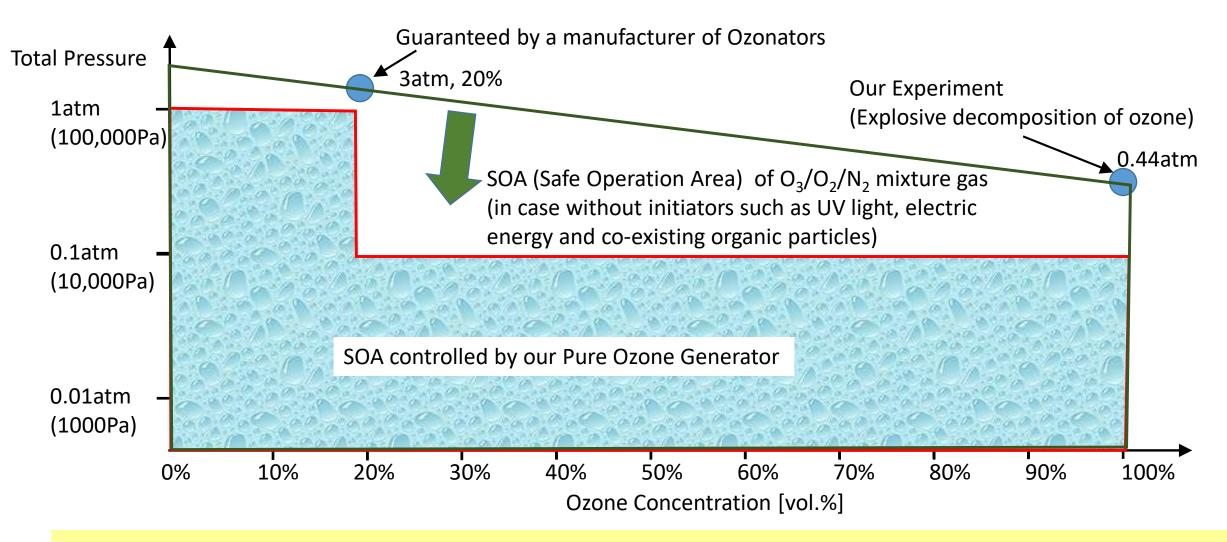
Throughout the operation time, ozone gas concentration and pressure are monitored and controlled so as to keep them inside the red area above! (No need to care for users)
