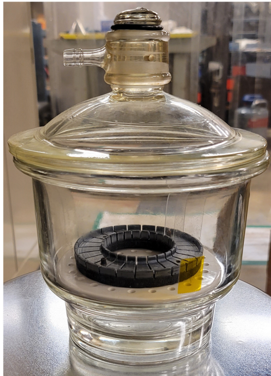
Fig. 2 Glass bell jar used in HTHH testing. Once prepped, the jar would be sealed with high-temperature vacuum grease and then be placed inside an oven.
