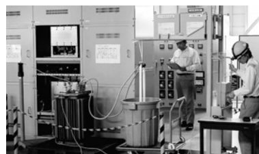
Fig. 2 Example of Artificial Ground Fault Testing Executed by a Conventional Method (Real ground fault simulation on load side)
